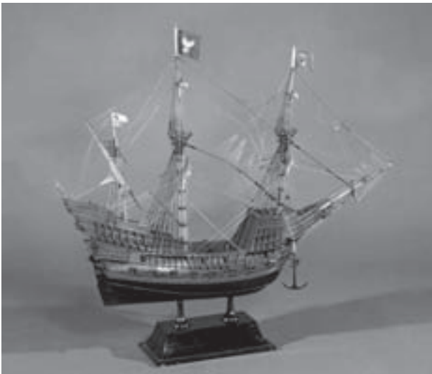
A model of the “Smok” – one of the earliest galleon type ships on the Baltic constructed in years 1570-1572 by two Venetians in Elblag (Elbing) for the order of the Polish king Zygmunt August. Photo Ewa Meksiak.
