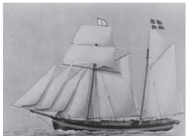
The ship “Balder” from Marstal (Denmark) represents the galeas type of small trade vessel.
