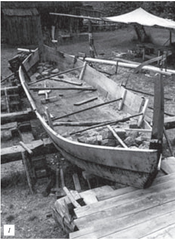
The different stages of the boatbuilding process of the Kurėnas boat at the Lithuanian Sea Museum in the summer of 2001. (pictures 1, 2, 3)
