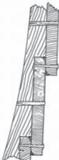
Typical overlapping sides planks observed in wrecks of the cog ships – clenches nails and the caulking compressed by battens stapled to the planks.
