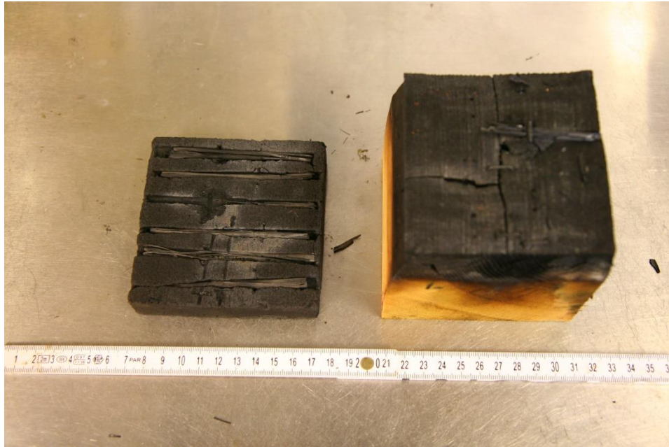
Figure 4.19 Removed plaster coat from the timber member after cooling down.
