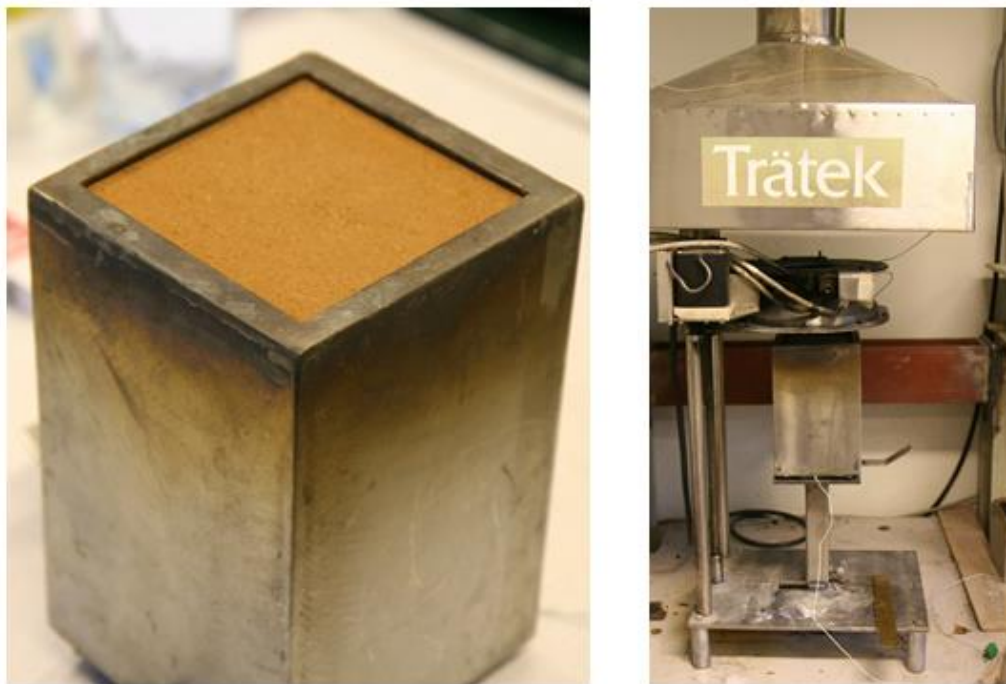
Figure 4.11 Fixed specimen and its position under the cone heater.
