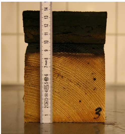
Figure A-4 Documentation after the test. Timber specimen with a 40 mm plaster.
