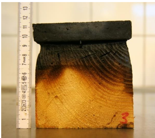
Figure A-2 Documentation after the test. Timber specimen with a 20 mm plaster.
