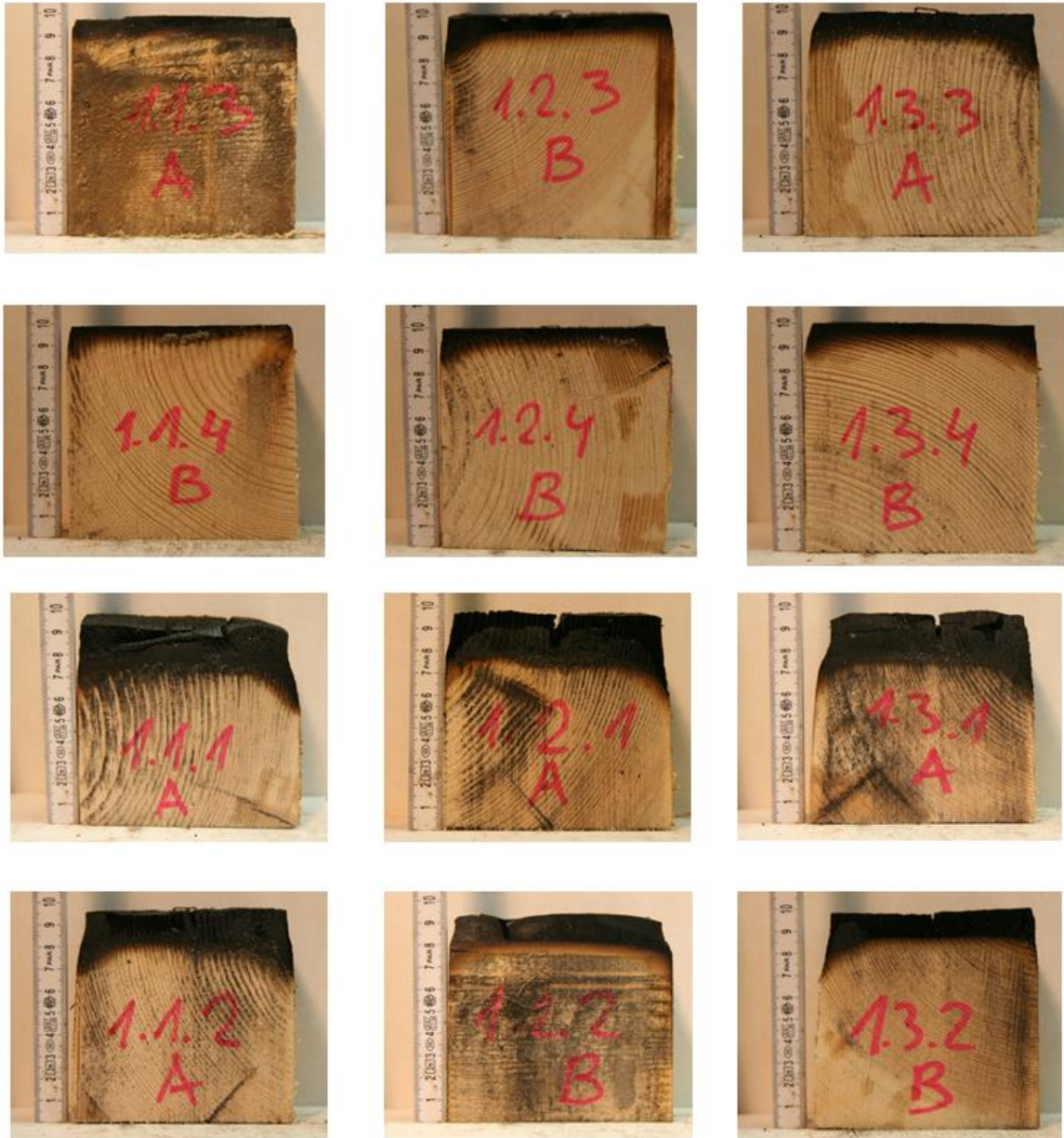
Figure 4.27 Documentation of residual cross-sections of timber member.
