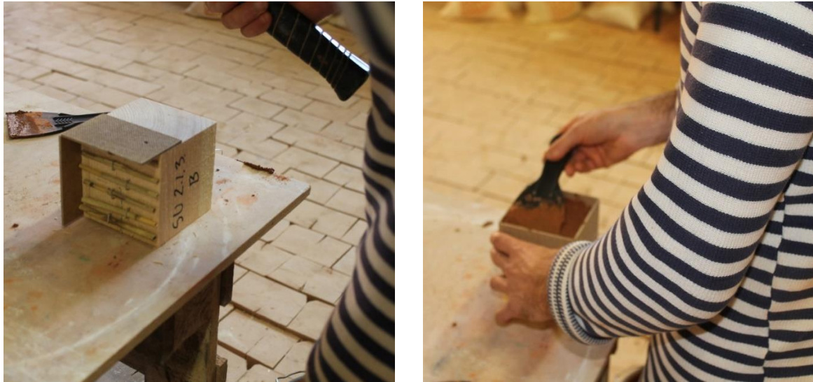
Figure 4.4 Installing the edge fixers and plastering the specimens.
