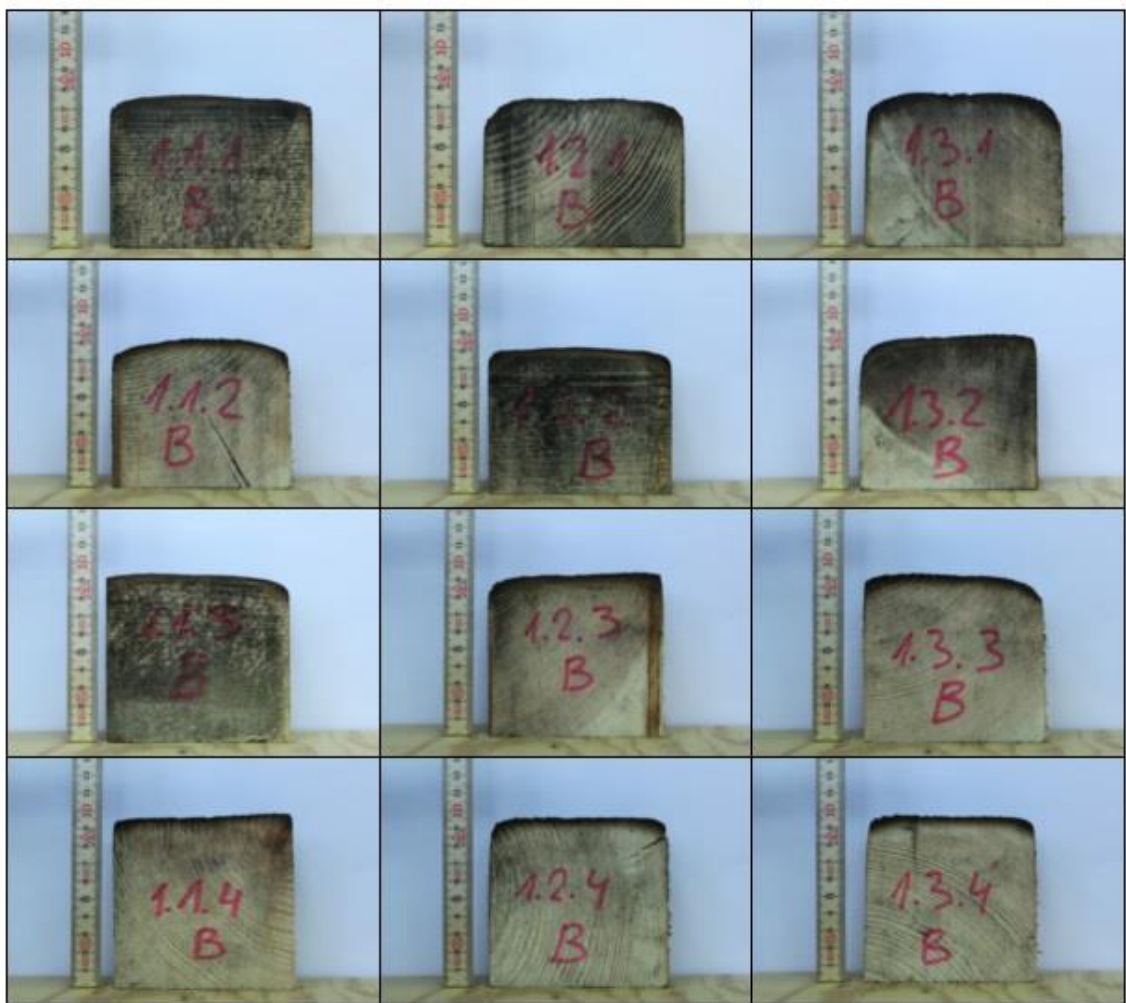
Figure B-2 Documentation of the residual cross-sections. Specimens variant B.
