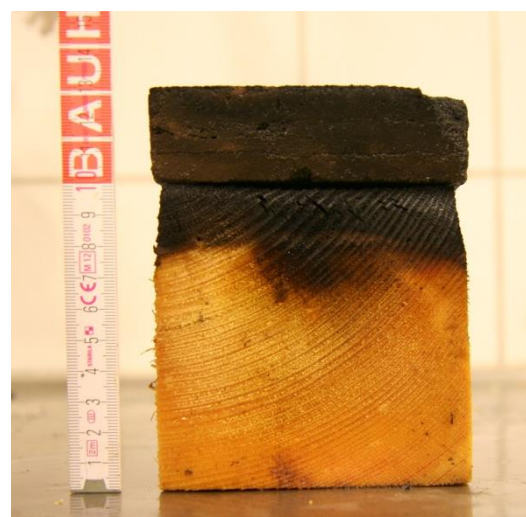
Figure A-3 Documentation after the test. Timber specimen with a 30 mm plaster.
