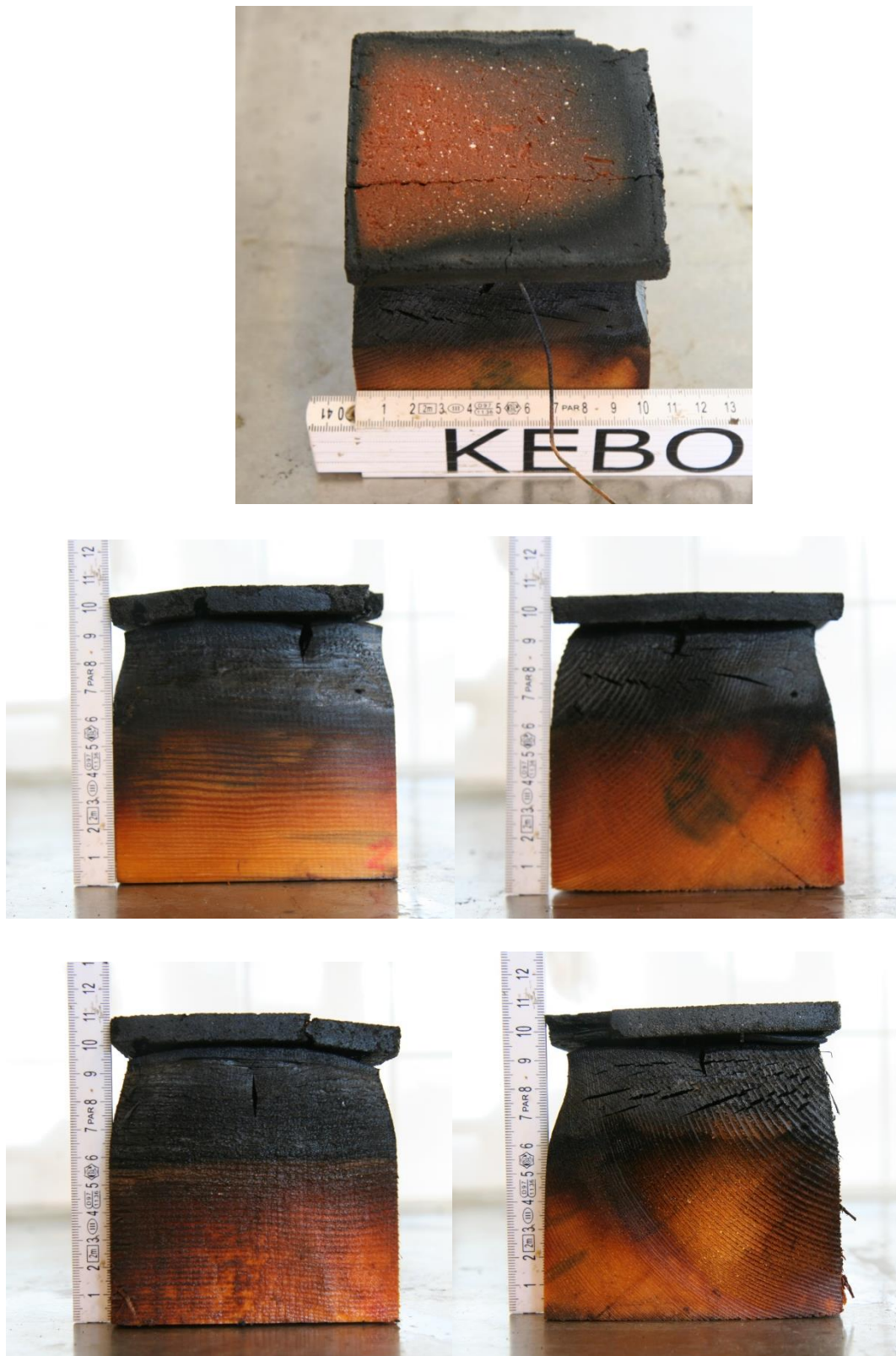
Figure A-1 Documentation after the test. Timber specimen with a 10 mm plaster.
