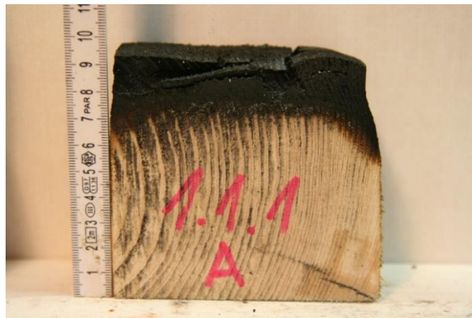
Figure 4.25 Timber specimen after cut in half.
