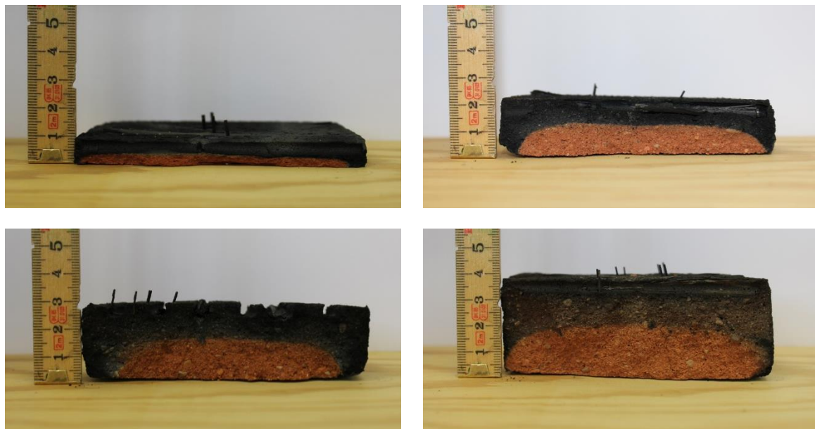
Figure 4.28 Documentation of the cross-sections of plaster after tests.
